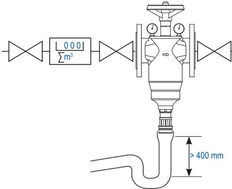
The untreated water flows through a stainless steel filter element in the Multipur filter. Foreign particles  $> 100 \mu\text{m}$  or  $> 200 \mu\text{m}$  are thus retained. Depending on their size and weight, these particles either fall directly into the lower part of the filter housing, or adhere to the filter element.
